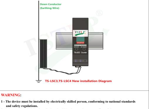
2 - It is recommended that installation should be done under power off condition.
